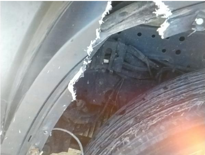
1: Qtr Panel Arch Extension ns Broken Replace
