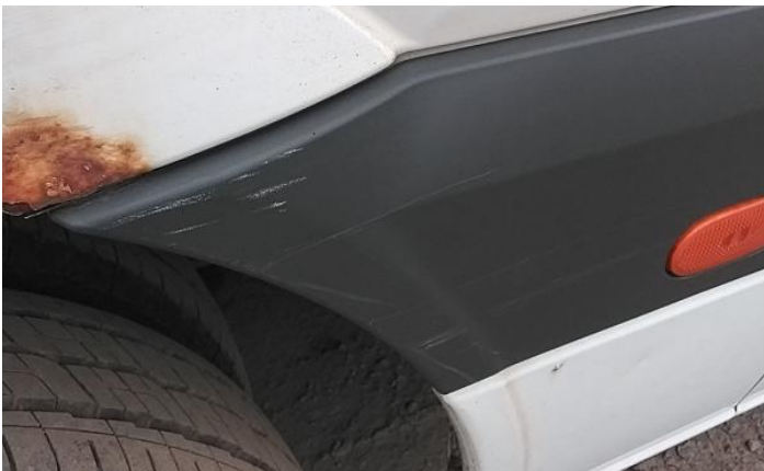
5: Panel Rear Chipped Multiple Chips
