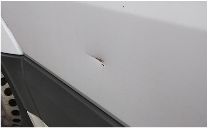
9: Qtr Panel osr Chipped Multiple Chips
