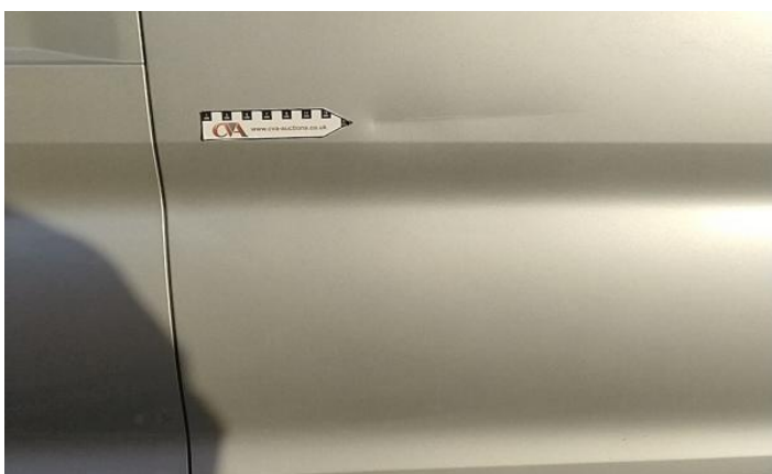
29: Qtr Panel osr Scratched Over 25mm Not Thru Paint
