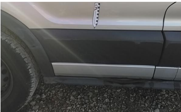
5: Moulding nsf Wing Scuffed (Unpainted) Over 100mm
