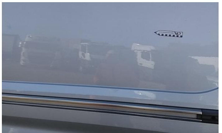
12: Door nsr Dented Between 10mm + 30mm
