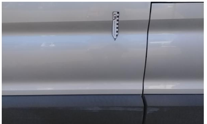
10: Door nsr Dented Between 10mm + 30mm
