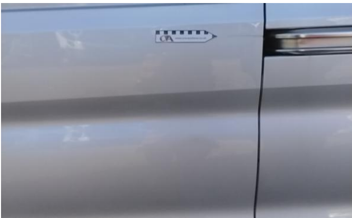
9: Door nsr Dented Over 30mm
