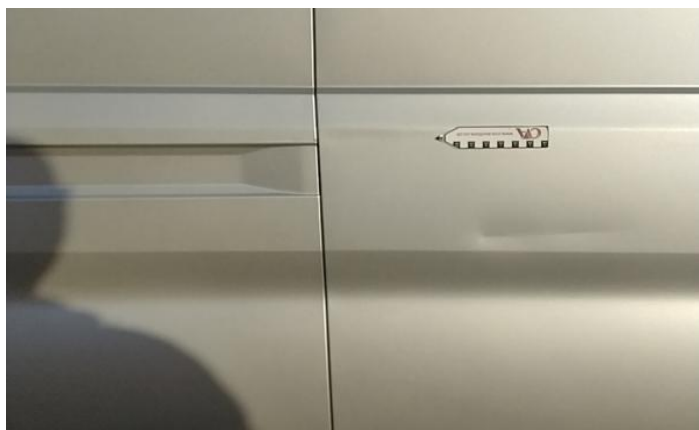
28: Qtr Panel osr Dented Over 30mm
