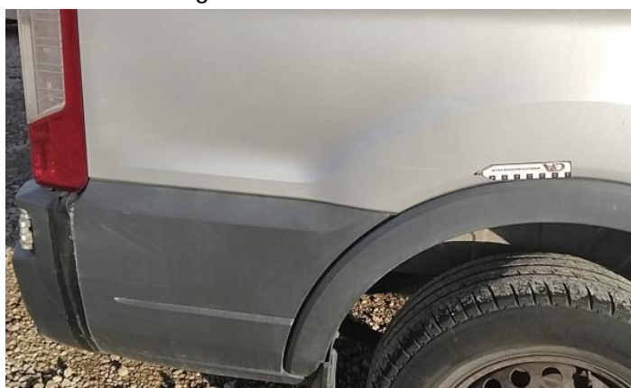
30: Qtr Panel osr Dented With Paint Damage
