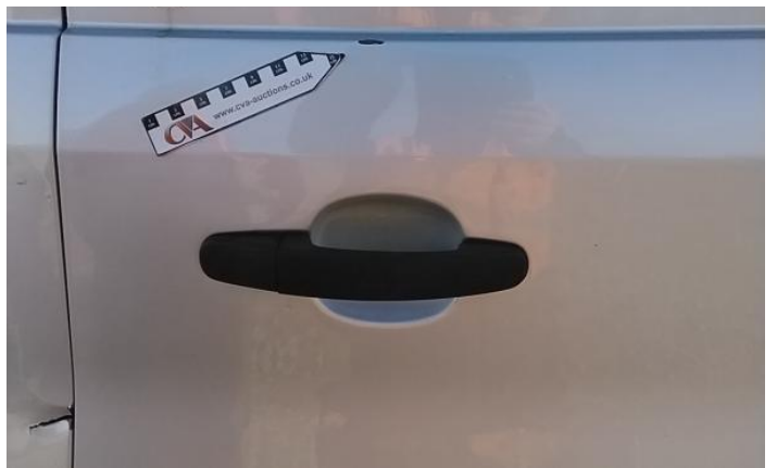
22: Door osr Dented Over 30mm
