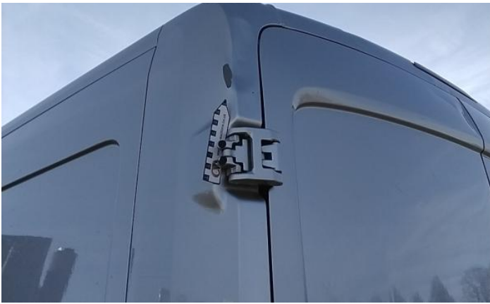
15: Qtr Panel Moulding ns Scuffed (Unpainted) Over 100mm
