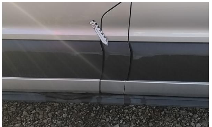
6: Door Moulding nsf Broken Replace
