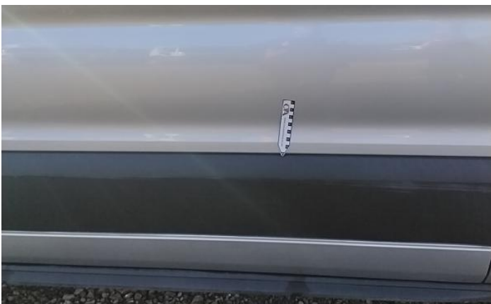
11: Door nsr Scratched Over 25mm Thru Paint
