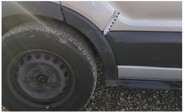
4: Bumper Front Moulding Scuffed (Unpainted) Over 100mm
