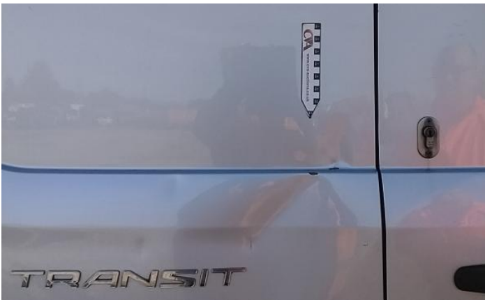
17: Qtr Panel nsr Dented With Paint Damage
