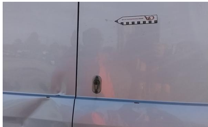
21: Door nsr Dented Over 30mm
