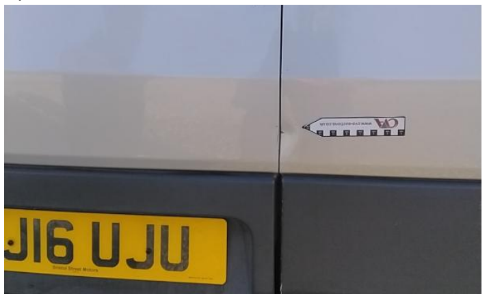
24: Door osr Scratched UpTo 25mm Thru Paint
