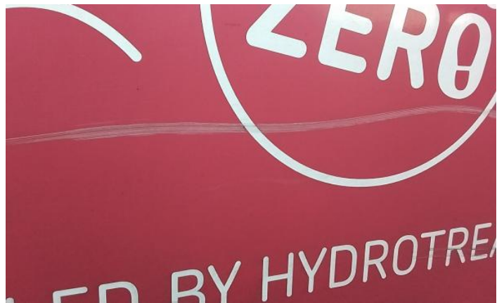
4: Door nsf Scratched Over 25mm Thru Paint
