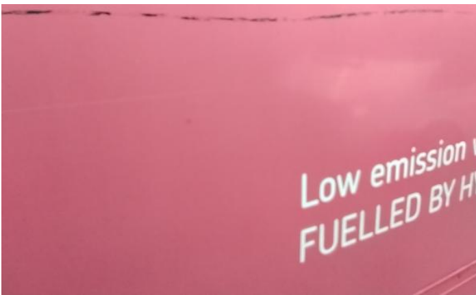
3: Door nsf Scratched Over 25mm Thru Paint
