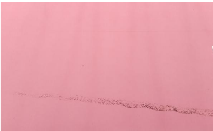
5: Qtr Panel nsr Scratched Over 25mm Not Thru Paint
