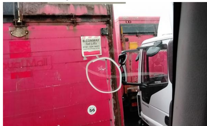
5: Door osf Dented With Paint Damage
