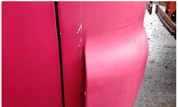
6: Door osf Scratched Over 25mm Thru Paint
