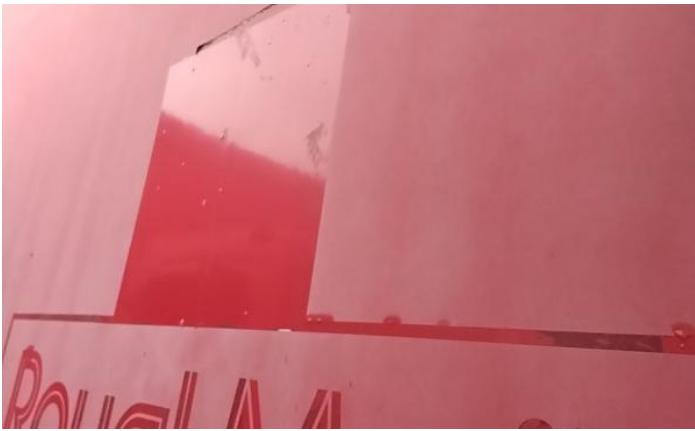
3: Wing nsf Scratched Over 25mm Thru Paint
