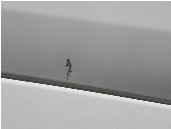
3: Door nsf Scratched Over 25mm Thru Paint
