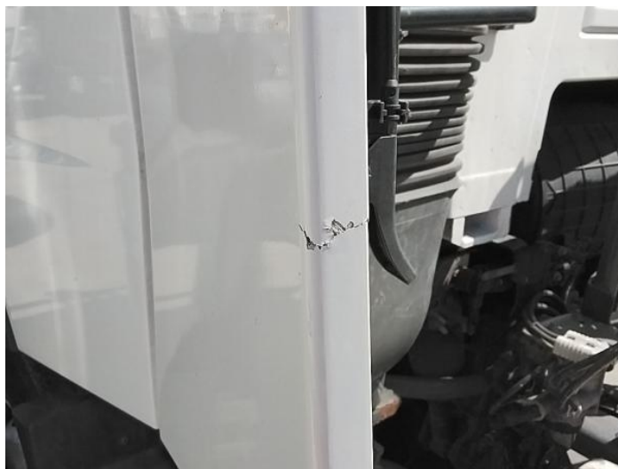
2: Panel Front Cracked Replace
