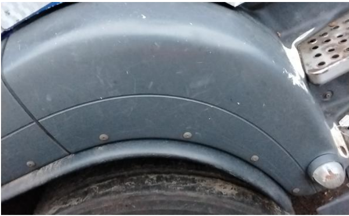
3: Wing nsf Scratched Over 25mm Thru Paint
