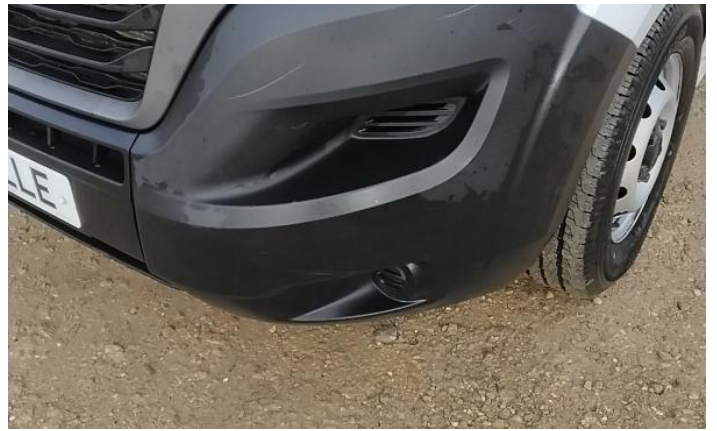
4: Bumper Front Moulding Scuffed (Unpainted) Over 100mm
