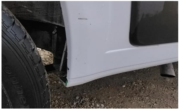
10: Door nsr Dented With Paint Damage
