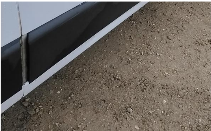
11: Qtr Panel nsr Dented With Paint Damage
