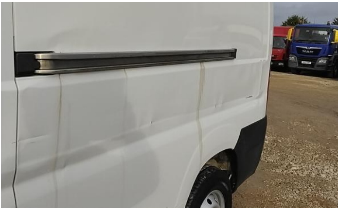
9: Door nsf Dented With Paint Damage
