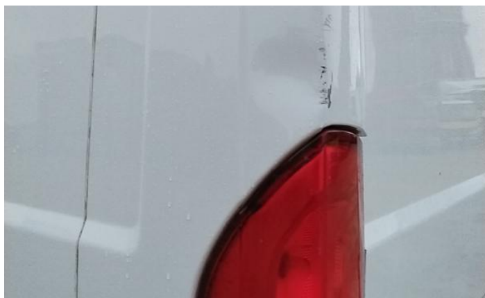
16: Qtr Panel Arch Extension ns Scuffed (Unpainted) Over 100mm
