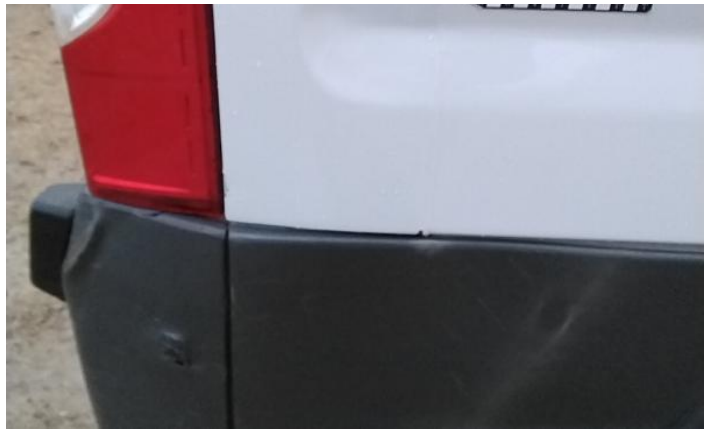
22: Bumper Rear Moulding Broken Replace
