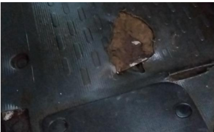
29: Sill os Rusted Over 5mm
