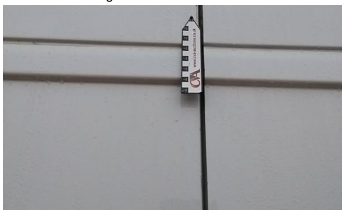
18: Qtr Panel nsr Dented With Paint Damage
