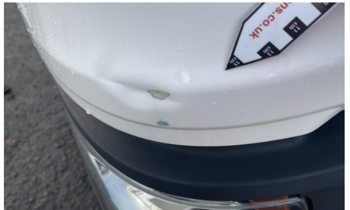
6: Qtr Panel nsr Rusted Over 5mm
