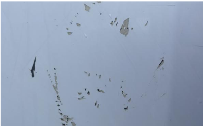
5: Qtr Panel osr Rusted Over 5mm
