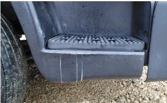
11: Panel Rear Scratched Over 25mm Thru Paint
