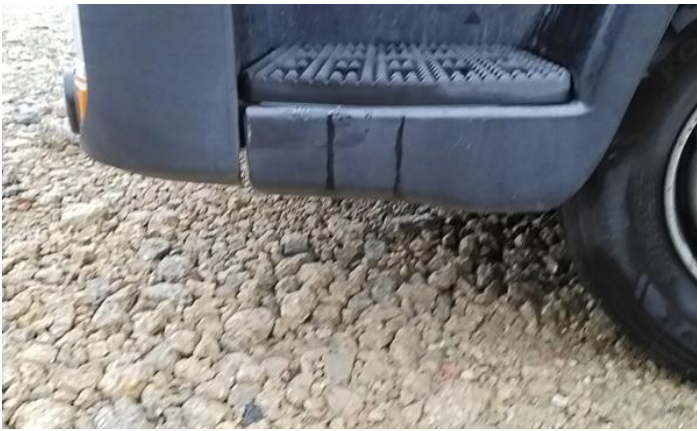
3: Bumper Front Hole Over 25mm
