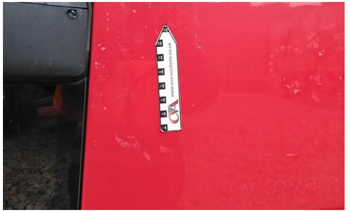
4: Wing nsf Scratched Over 25mm Thru Paint
