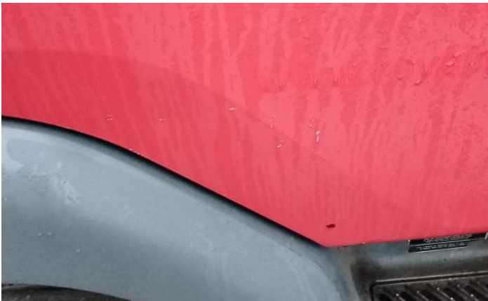
9: Qtr Panel osr Dented With Paint Damage
