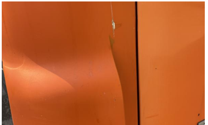
6: Qtr Panel nsr Dented Over 30mm
