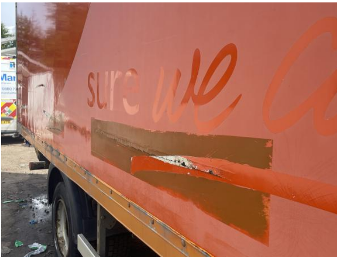
5: Qtr Panel osr Hole Over 10mm
