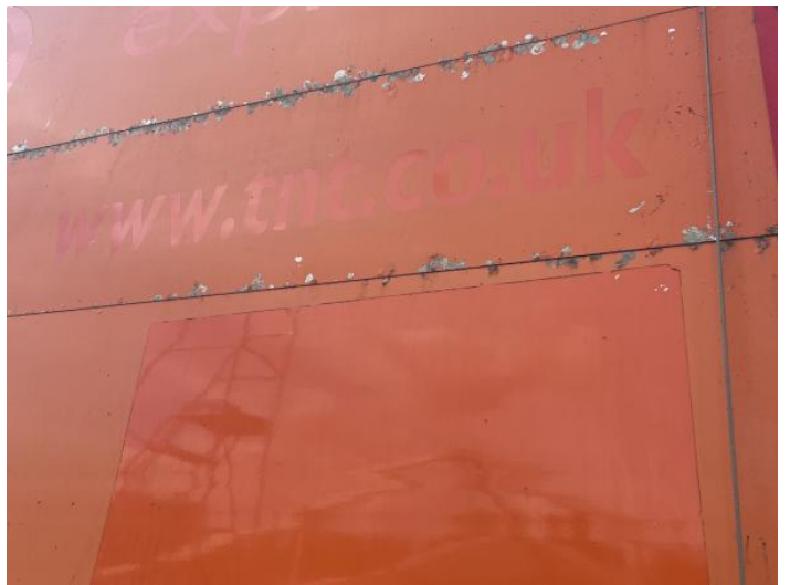
6: Tailgate Rusted Over 5mm
