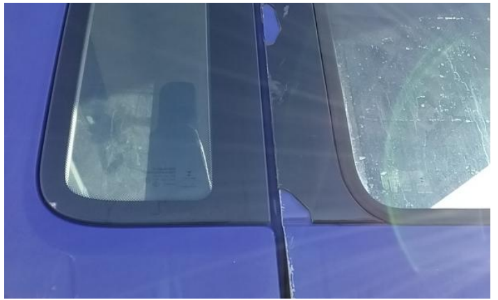
16: Door osf Scratched Over 25mm Thru Paint
