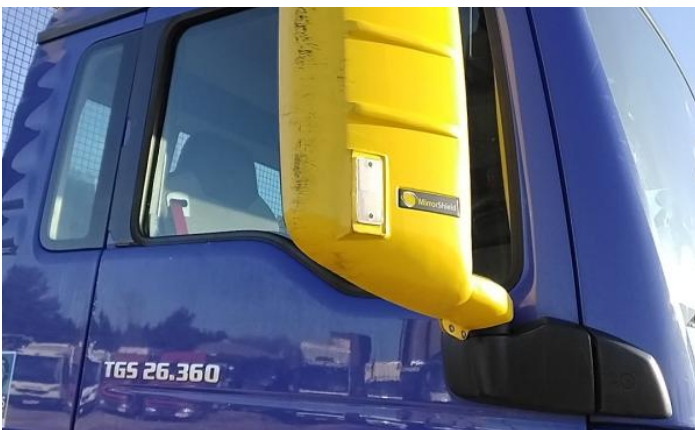
11: Door nsf Scratched Over 25mm Thru Paint
