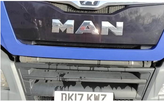
3: Bumper Front Moulding Scuffed (Unpainted) Over 100mm
