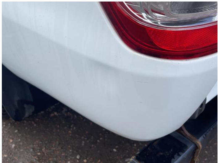
6: Qtr Panel nsr Dented Between 10mm + 30mm
