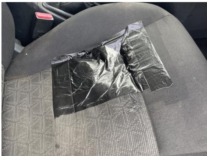
1: Seat Base Cover osf Torn Over 3mm
