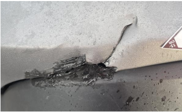
3: Sill os Rusted Over 5mm
