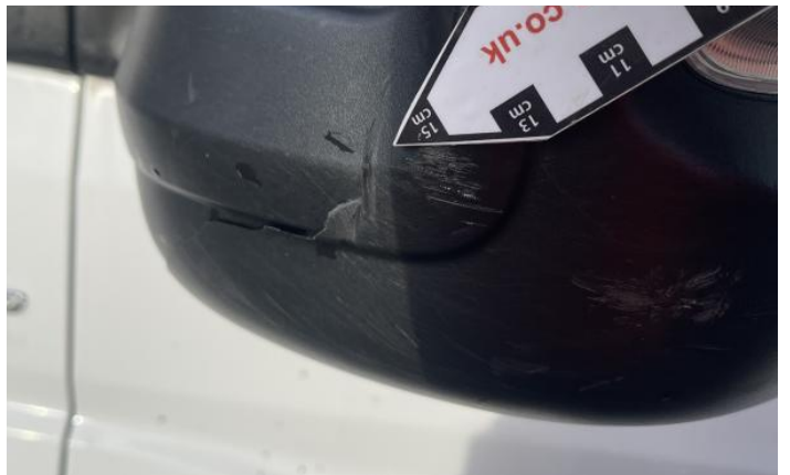
12: Door nsf Dented Over 30mm
