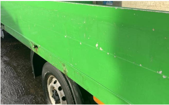
9: Qtr Panel osr Rusted Over 5mm
