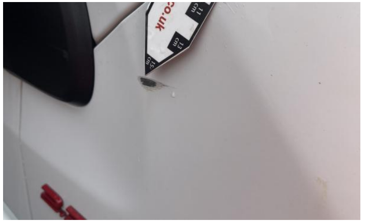
4: Bonnet Dented Over 2 UpTo 10mm
