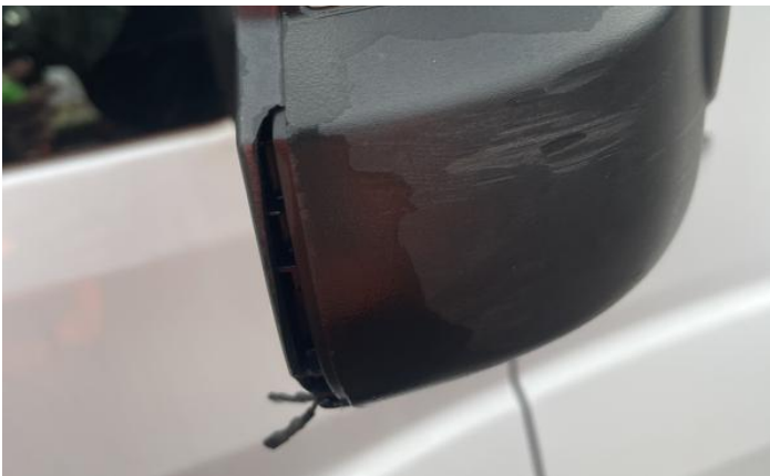
5: Bumper Front Moulding Broken Replace
