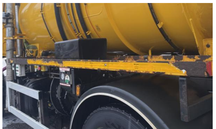
6: Qtr Panel osr Rusted Over 5mm
