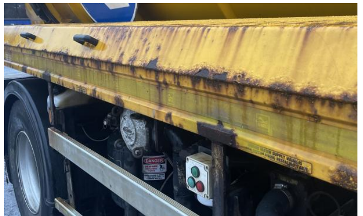
4: Wing osf Cracked Replace
