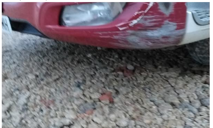
6: Wing nsf Chipped Multiple Chips
