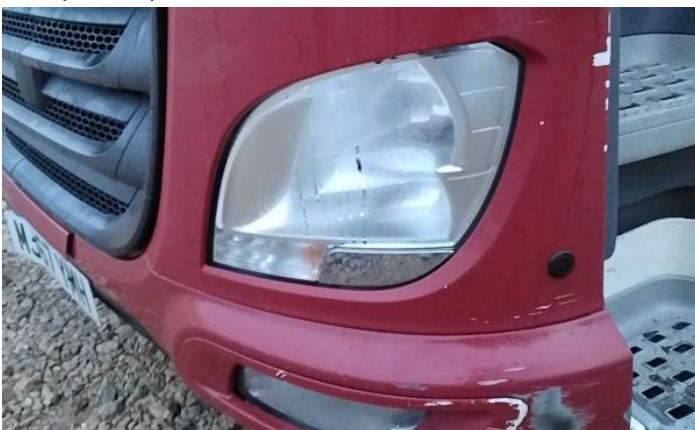
5: Bonnet Chipped Multiple Chips
